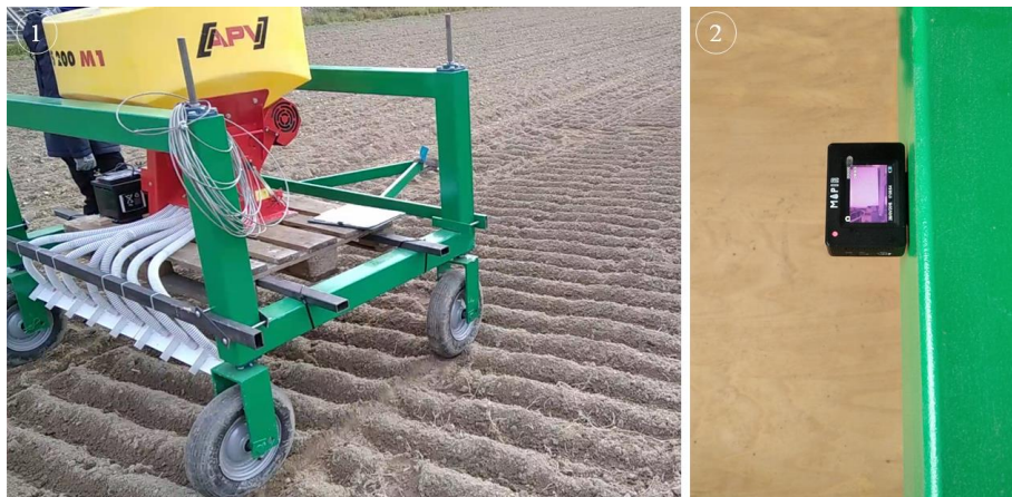
Fig. 2. Funicular system in the experimental layout: 1 – trolley equipped with a pneumatic seeder; 2 – RGB/IR camera attached to the side of the frame
