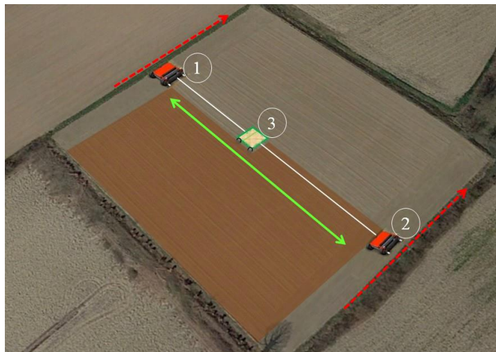
Fig. 1. Schematic representation of the developed system: 1 and 2 – machinery at the opposite headlands of the field, moving along the slow movement directions (as indicated by the red dotted arrows); 3 – trolley, alternatively moving back and forward (as indicated by the green arrow direction)
